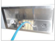
Back panel with net input, air input, air's manometer for Ø6x8mm Rilsan tube and pressure regulator.
