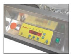
Frontal panel with emergency stop button, control keyboard and net switch.
